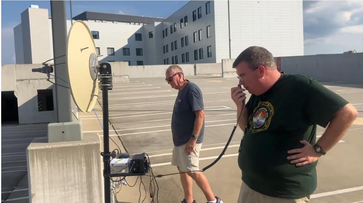
My first 10 GHz setup in August 2025 with IC-705, DEMI low-power 10 GHz transverter, non-functional 1-watt amplifier, and 2-foot dish with dual-band feed -- that I couldn't see over to aim! (K4CNY photo)
